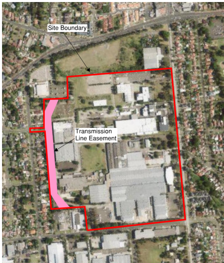
Figure 6 – Location of Overhead Transmission Line Easements
